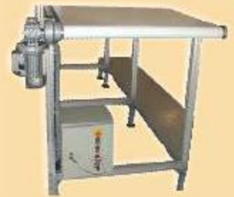
CONTROL PANEL WITH CONTACTOR, ON -OFF SWITCHES & VFD
