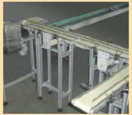
Blister Turning Conveyor
